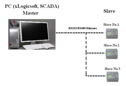
At present xLogic supports baud rate: 9600. The default is 9600. The default is non parity checking mode. MODBUS RTU is used as communication protocol of xLogic. The defaulted communication protocol is MODBUS RTU format .Defaulted address: 1, and legal address range: 1~247.
